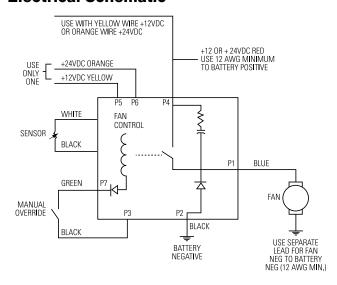
NOTE: This switch should be fused to prevent damage if ground is lost. A 30 amp fuse is required in the power supply.
